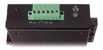
The image on the left details the case of an Industrial Ethernet Switch that acts as the heat sink for the unit. The image on the right shows dual power inputs as well as a dry contact for connecting alarm devices for visual or audio warning in the event of a power supply failure.
