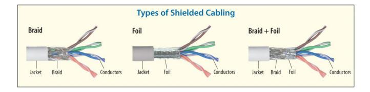
When building a shielded cable plant it is important to use shielded cable, shielded connectors and shielded interconnection points such as patch panels in order for the shielding to be effective against EMI/RFI. Additionally, proper bonded grounding of all components is crucial to attaining effective shielding.
