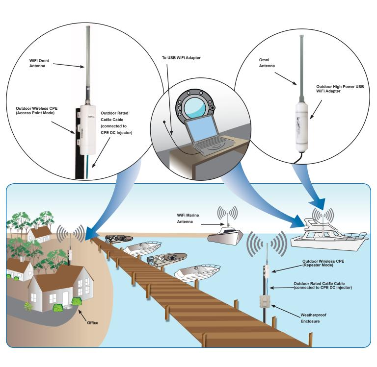
This diagram is representational only and depicts a typical Marina WiFi application. Each wireless installation is unique and results can vary due to many different environmental factors. For outdoor wireless networks Line of Sight (LOS) must be considered. Basically that means you will need a clear unobstructed view of the antenna from the remote point in the link. Trees and leaves are obstructions to 802.11 frequencies so they will partially or entirely block the signal.
