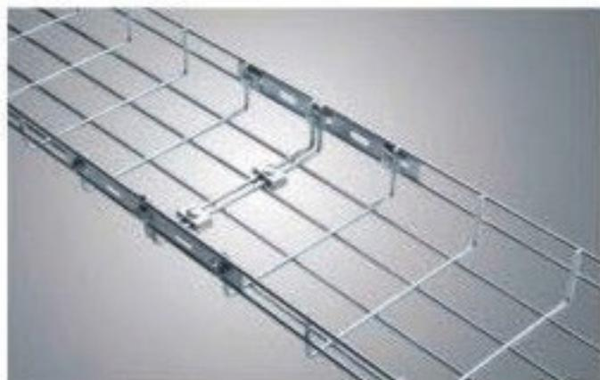
**PART NO.:** LC-CSB**DESCRIPTION:** CORNER STRENGTH BAR**Application:** Make T and Cross connectors.**Fit for:** Diameter of wire from 3.5mm to 6.0mm**Includes:** Bar x 1, KK34-top x 4, M6 x 20bolt x 4, M6 Nut x 4**Features:** (1) Very Strong Connection;
