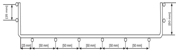
**LCM10 Wire Mesh Cable Tray - Nickel Plated**
