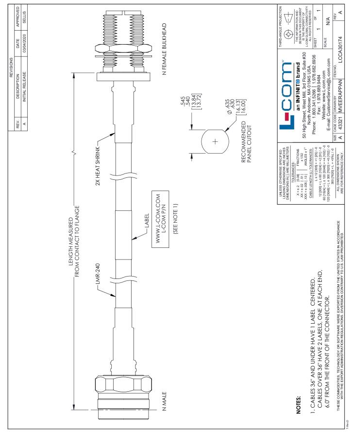
LCCA30174-FT4 REV 1.0 | © 2019 Infinite Electronics, Inc. L-com is a registered trademark of Infinite Electronics, Inc.
