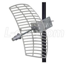
This antenna is supplied with a tilt and swivel mast mount kit. This allows installation at various degrees of incline for easy alignment. They can be adjusted up or down from 0° to 60°.
