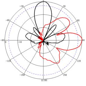
Freq:5400MHz Date:2014-03-10 Elevation:H-plane Polar-Across:Main Polarization:Vertical Max:-23.98dB HPBW(3dB):21.89° FBR:26.37dB
