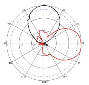
Freq:2400MHz Date:2014-03-10 Elevation:H-plane Polar-Across:Main Polarization:Vertical Max:-16.19dB H-PBW(3dB):43.94° FBR:28.09dB
