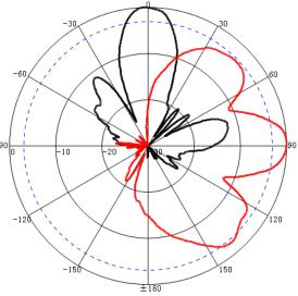
Freq:5850MHz Date:2014-03-10 Elevation:H-plane Polar-Across:Main Polarizion:Vertical Max:-27.61dB HPBW(3dB):20.54\* FBR:26.75dB
