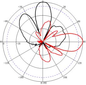
Freq:5400MHz Date:2014-03-10 Elevation:H-plane Polar-Across:Main Polarization:Horizonta Max:-24.12dB HPBW(3dB):20.56° FBR:23.99dB
