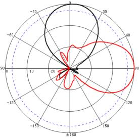
Freq:2450MHz Date:2013-01-16 Elevation:H-plane Polar-Across:Main Polarization:Vertical Max:-11.59dB HPBW(3dB):43.36\* FBR:28.49dB
