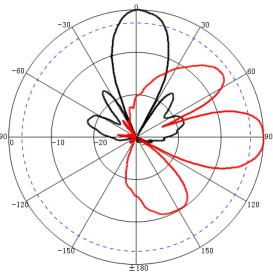
Freq:5500MHz Date:2013-01-16 Elevation:H-plane Polar-Across:Main Polarizion:Vertical Max:-21.33dB HPBW(3dB):22.90° FBR:28.68dB
