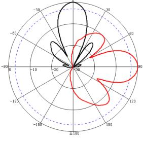
Freq:5125MHz Date:2013-01-16 Elevation:H-plane Polar-Across:Main Polarization:Vertical Max:-16.90dB HPBW(3dB):22.48° FBR:33.93dB
