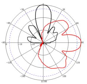
Freq:5875MHz Date:2013-01-16 Elevation:H-plane Polar-Across:Main Polarization:Vertical Max:-24.67dB HPBW(3dB):22.64\* FBR:28.88dB
