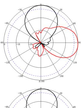
Freq:2400MHz Date:2013-01-16 Elevation:H-plane Polar-Across:Main Polarization:Vertical Max:-12.16dB HPBW(3dB):46.78° FBR:27.00dB
