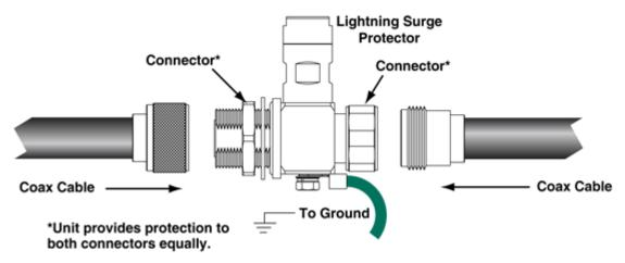
**Operational Note:** This 1/4 wave protector is not for use with coaxial cables carrying a DC voltage such as in the case of a remote-mounted amplifier or LNA. For applications requiring DC capability please see our Gas Tube coax protectors.
