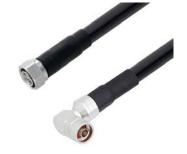
Low Loss 4.3-10 Male to N Male Right Angle Cable Assembly using LMR-600 Coax, 2 FT with Times Microwave Components
