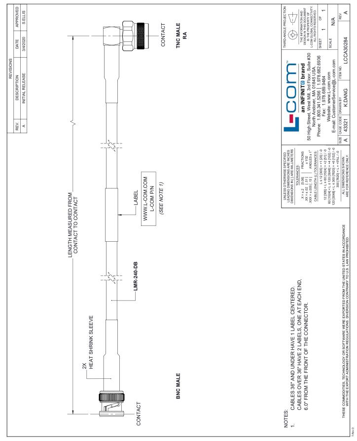
LCCA30284-FT6 REV 1.0 | © 2019 Infinite Electronics, Inc. L-com is a registered trademark of Infinite Electronics, Inc.
