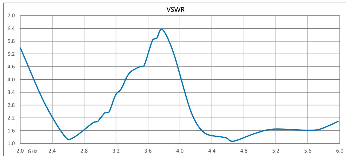
Embedded 2.4/5 GHz PCB Antenna, 4 dBi gain, IPEX Connector
