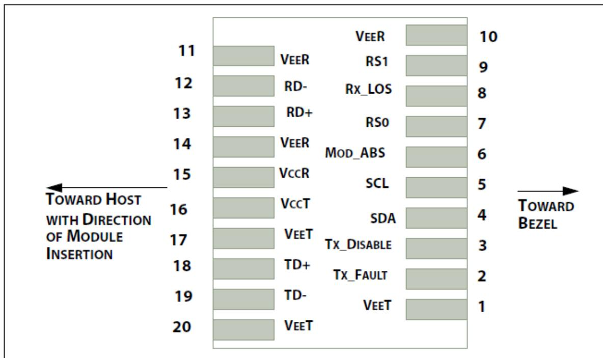
Fiber Optic Transceiver, SFP+, RJ-45, Copper
