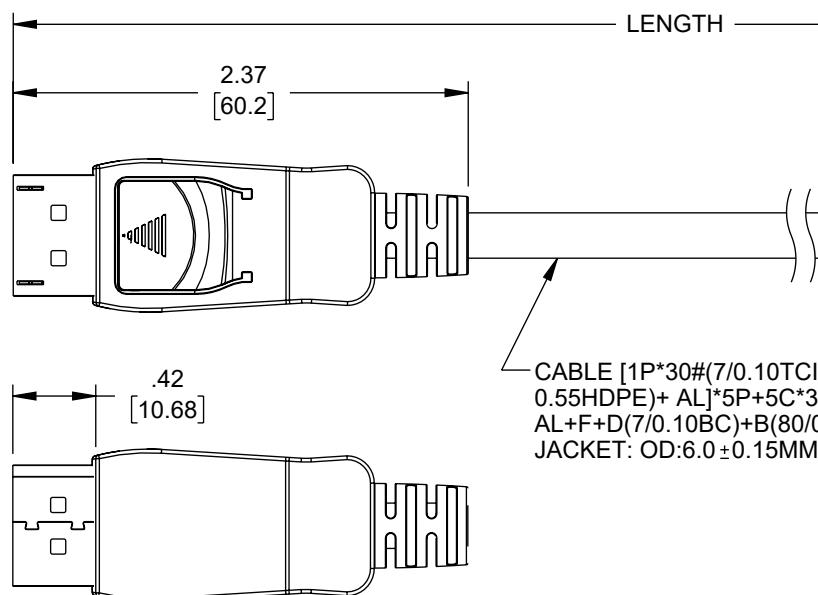
CABLE [1P\*30#(7/0.10TCID:0.78MM-FM-PE)+D(7/0.10TCID:0.55HDPE)+ AL]\*5P+5C\*30#(7/0.10TCID:0.55HD-PE)+ AL+F+D(7/0.10BC)+B(80/0.12AM)
