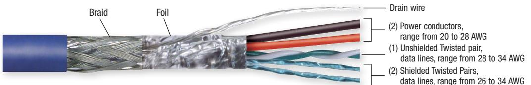
USB 3.0 adds two shielded data pairs to the USB 2.0 cable specifications. This addition allows for the faster performance in downloading data or video. Similar concept to changing a 2 lane highway to a 6 lane highway - much more traffic can pass through!
