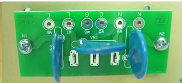
Built-In Surge Protector on Back side of Plate
