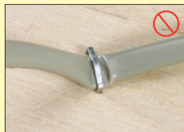
DO NOT use a stapler for installations
