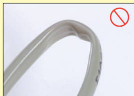
DO NOT bend cable greater than 90 degrees
