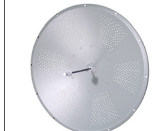
HG5833D - Perforated holes in the 900mm diameter dish antennas help reduce wind loading.
