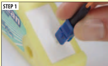
STEP 1 Softly press fiber tip in cleaning window using a figure 8 motion.
