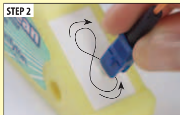
STEP 2 Repeat 3 times, inspecting fiber tip for cleanliness.
