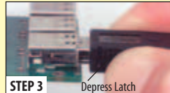
STEP 3 To remove the latching USB connector, simply depress the release mechanisms on the sides of the backshell and pull apart.
