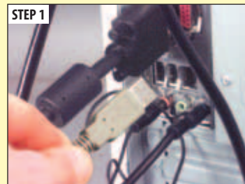
STEP 1 Simply connect the mountable extension cable once to the USB port on the back of your computer.
