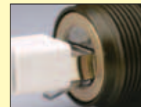
EMC Shroud (rear view) – conductive surface with shielded cable
