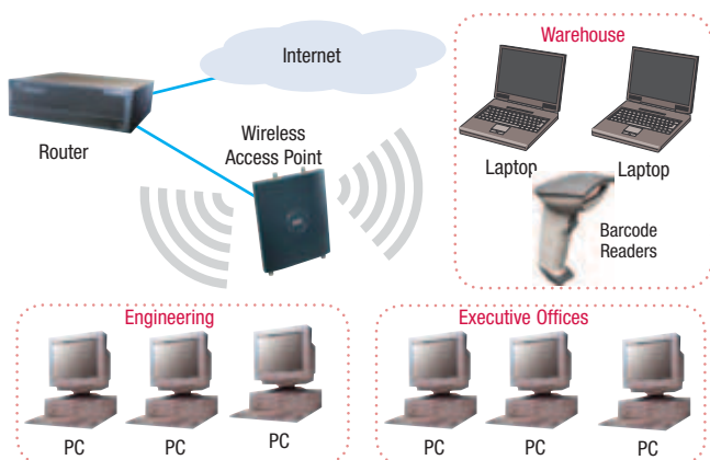
The diagram below shows a typical business wireless LAN.
