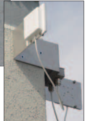
HG-2414P Flat Panel Antenna shown below
