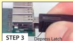
STEP 3 To remove the latching USB connector, simply depress the release mechanisms on the sides of the backshell and pull apart.
