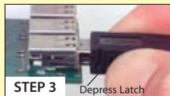
STEP 3 To remove the latching USB connector, simply depress the release mechanisms on the sides of the backshell and pull apart.
