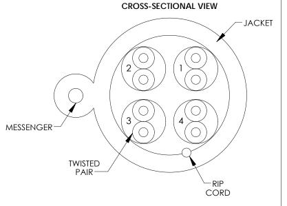
CAT5e, UTP, OUTDOOR RATED CABLE WITH MESSENGER, 4 TWISTED PAIR 24AWG SOLID-BARE COPPER
