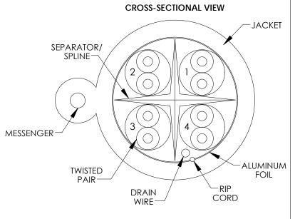
CAT6 550MHz, F/UTP, OUTDOOR RATED CABLE (SHIELDED) WITH MESSENGER, 4 TWISTED PAIR 23AWG SOLID-BARE COPPER
